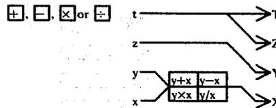
Look at the contents of the stack as we calculate  $(3 \times 4) + (5 \times 6)$ . Directly above the keys pressed you see the information in X, Y, Z and T after the keystroke.
